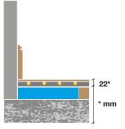
Heat output of up to 75 watts/m<sup>2</sup>
